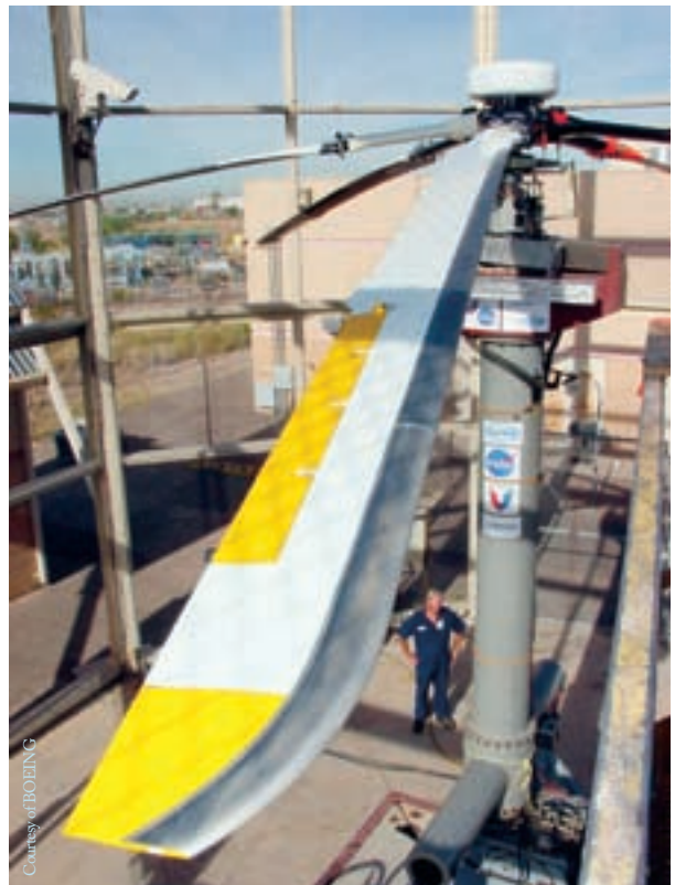
Figure 3: Whirl tower testing of smart rotor. 18
