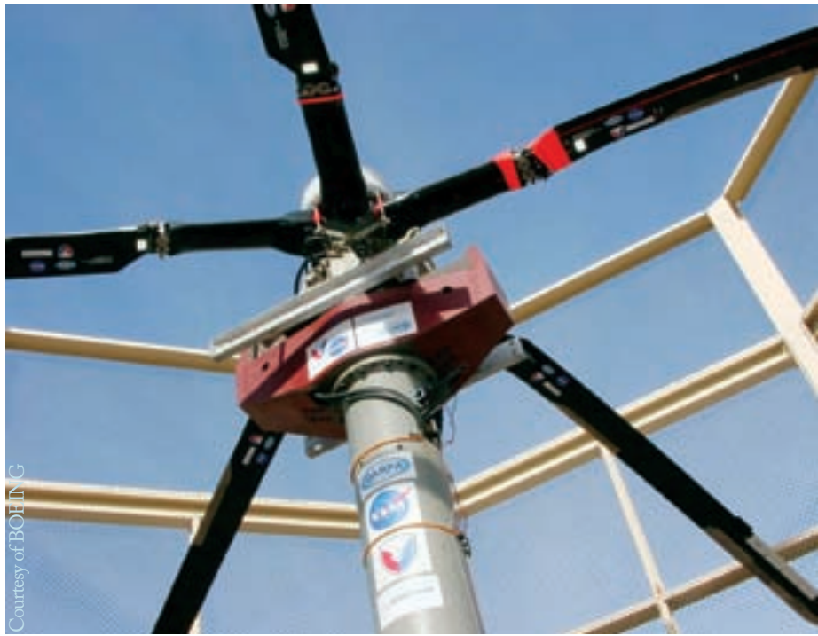
Figure 4: Whirl tower testing of smart rotor.
