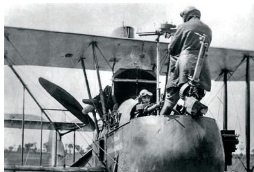
Photo demonstrating the observer's firing positions in the Royal Aircraft Factory FE2d. The observer's cockpit was fitted with three guns, one fixed forward-firing for the pilot to aim, one moveable forward-firing and one moveable rear-firing mounted on a pole over the upper wing. The observer had to stand on his seat in order to use the rear-firing gun.
